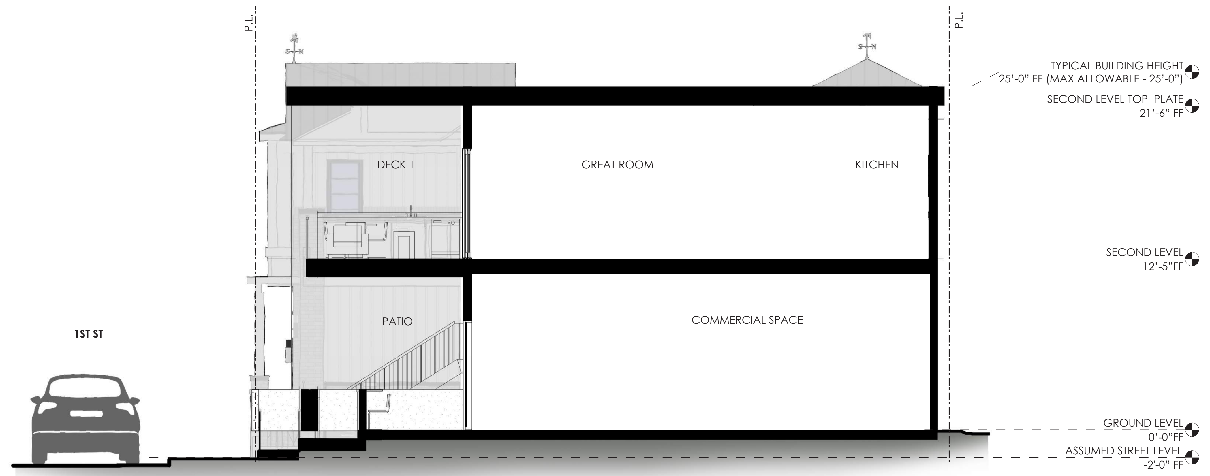
1 SHORT SECTION LOOKING NORTHWEST 1/4" = 1'-0" (24 X 36 SHEET)
