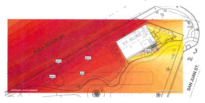
The first sound wall acoustic model below shows a 4 foot-high sound wall at the northwest property boundary line, adjacent to the sidewalk. Site sound levels are reduced from 65 dBA to 57 dBA.
