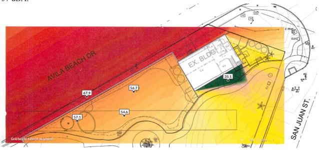
A six-foot wall is substituted in the acoustic model shown below. Incremental sound level improvement is shown in the critical activity area.
