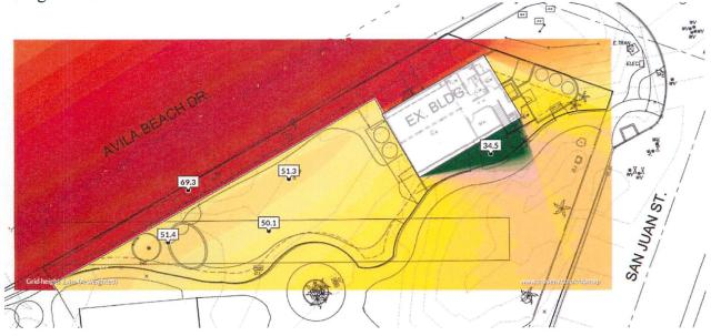
The final acoustic model considers a 6-foot high wall at the sidewalk / property boundary, with the added enhancement of lowering the overall site elevation by two feet. The total effective height of the sound wall is therefore equivalent to an 8 foot wall at the boundary. The resulting sound levels are shown below.
